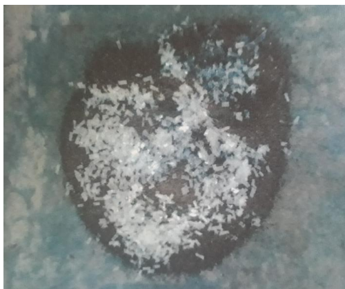
Fig.1. Reinforced Soil sample preparation
