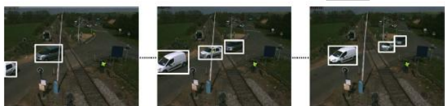
Figure 2: Tracking Process: From Right To Left
