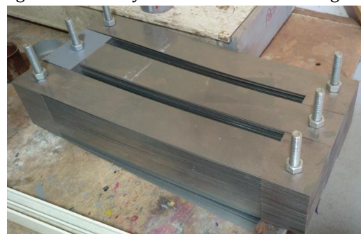
Figure 6: Core assembly of linear Autotransformer
