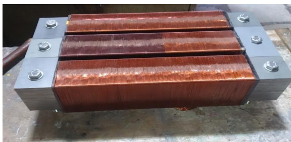
Figure 7: Copper winding on Bakelite bobbin
