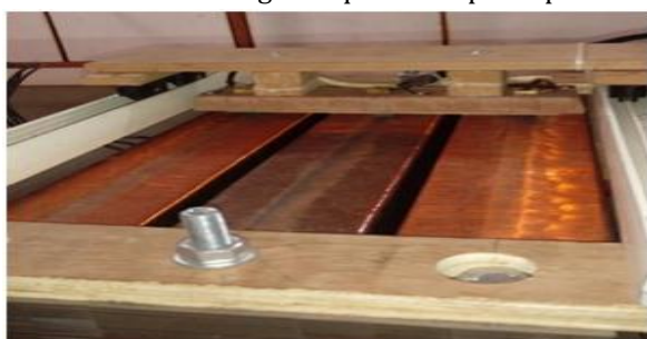
Figure 8: Brush holder and sliding mechanism
