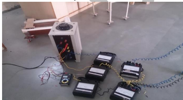
Figure 9: Testing of three phase autotransformer
