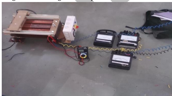
Figure 10: Testing of three phase linear autotransformer
