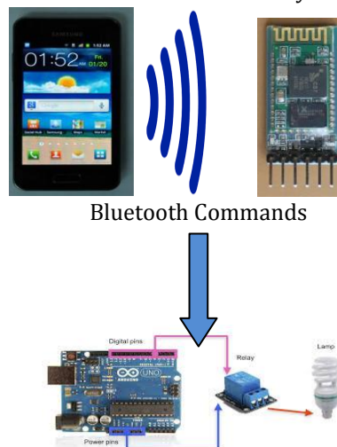
Arduino and relay connection Figure 3.1 Block diagram of the system
