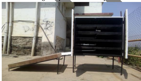
Fig.4 Experimental setup showing Trays & Ducts
