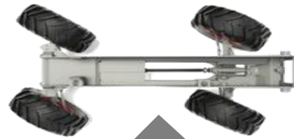
Fig.3.1 Crab steering mechanism
