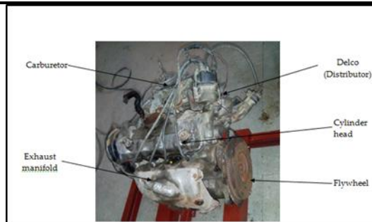
(Figure. 1 Maruti Esteem 4 cylinder petrol engine)
