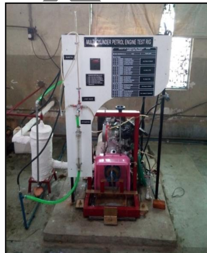
( Figure 18. Actual fabricated & erected test rig )
