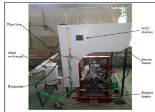
(Figure 14. Preplanned arrangement of all equipment and name plate before Mfg )
