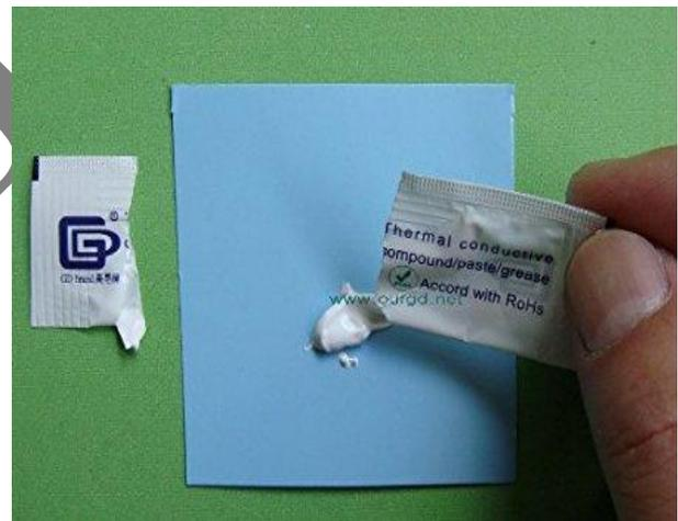
Figure 3 Thermal Grease
