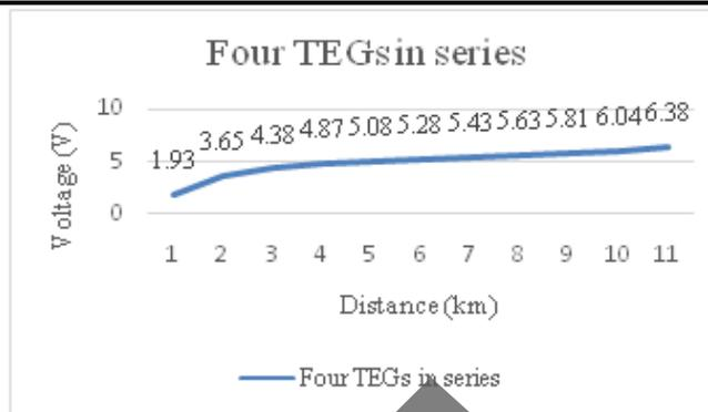
Figure 7 Graph of performance of four TEGs in actual setup
