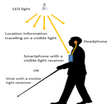
Figure 2 Indoor Navigation system for Visually Impaired using VLC
