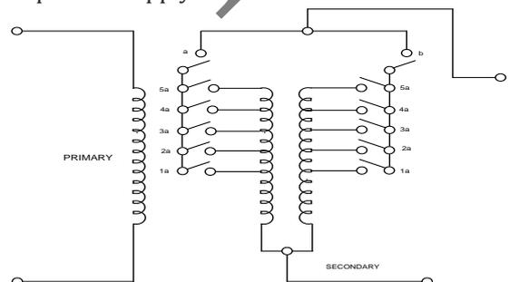
Fig.2: On-load tap-changing transformer
