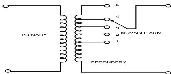
Fig.1: Off load tap changing transformer
