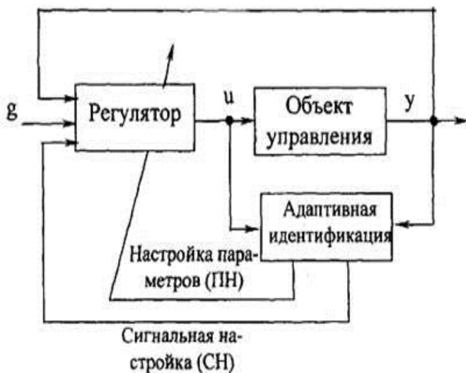
Figure: 2. An adaptive system with a parallel tunable model.
