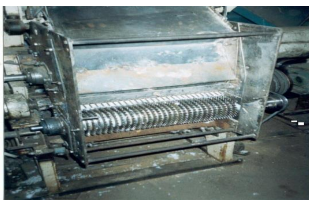
General View of the Bench Saw Installation Gin with a Throwing Drum
