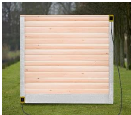
Fig. 3. Placement of the accelerometers
