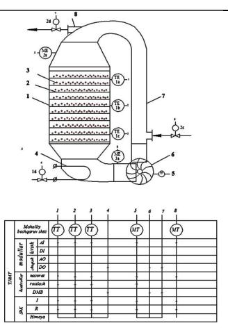
Figure 1. Automated functional scheme of acoustic-convective drying apparatus
