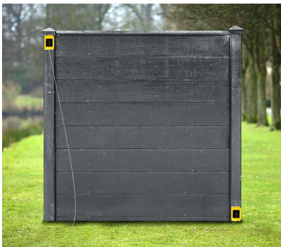
Fig. 3. Layout of the accelerometers on the terrace wall
