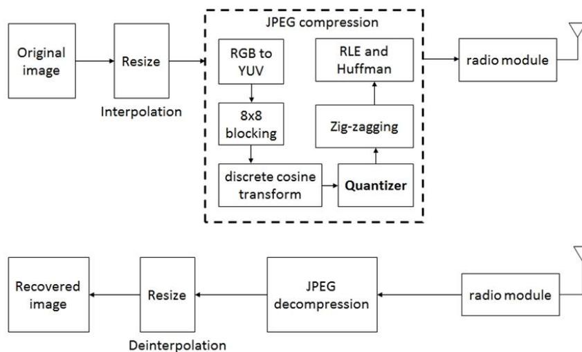
Figure 1. Framework of two-stage compression based low bandwidth video transmitter
