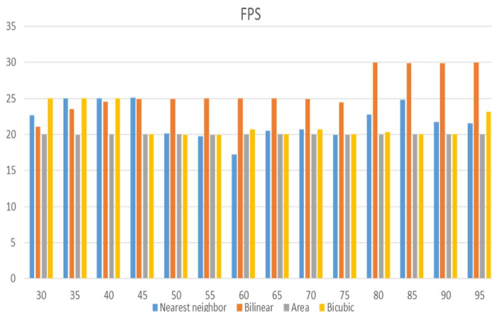
Figure 3. Comparison of the interpolation methods through FPS and quality
