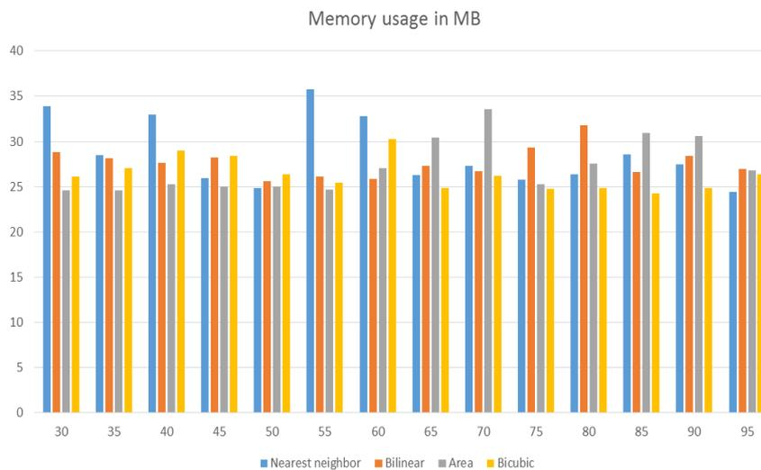
Figure 5. Comparison of the interpolation methods through RAM usage and quality
