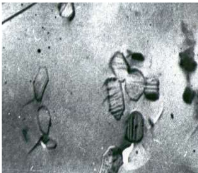
Picture 1. Type of stone of alkaline cement composition "slag + liquid glass" with an increase of 5000 times
