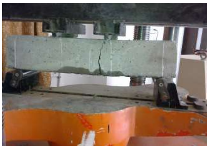
Fig. 1 - Flexural Test Setup
