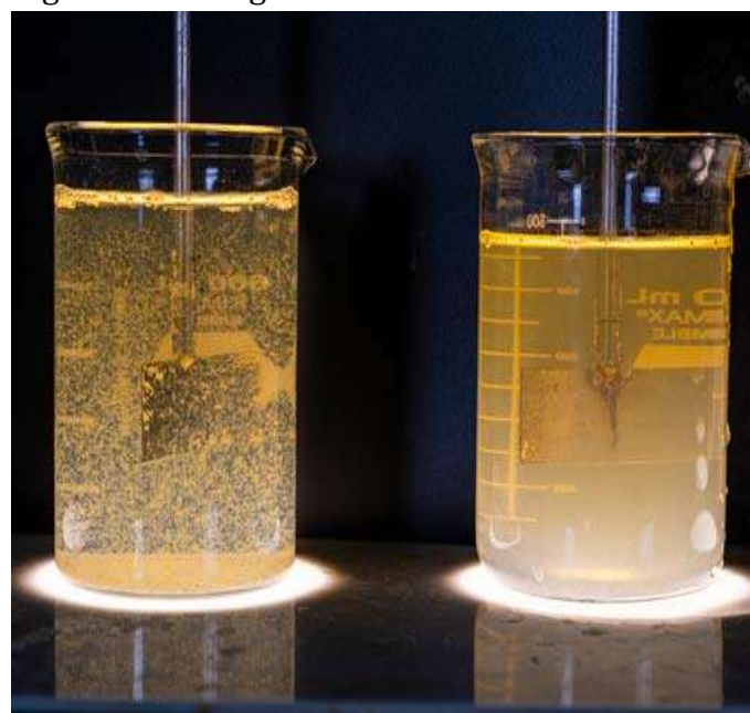
Figure 2: Results of laboratory testing of coagulant in water treatment plant Although coagulation cannot capture all the smallest organisms and viruses, it is an
