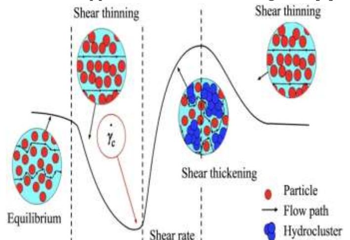
Figure 2: The shear thickening fluid behavior [7].
