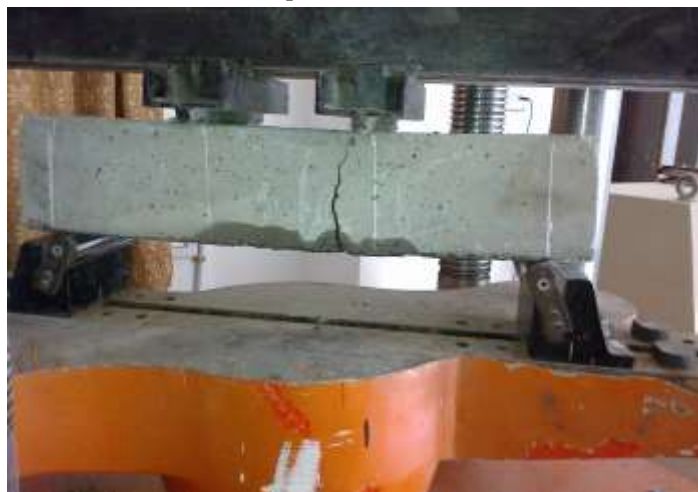
Fig. 1 - Flexural Test Setup
