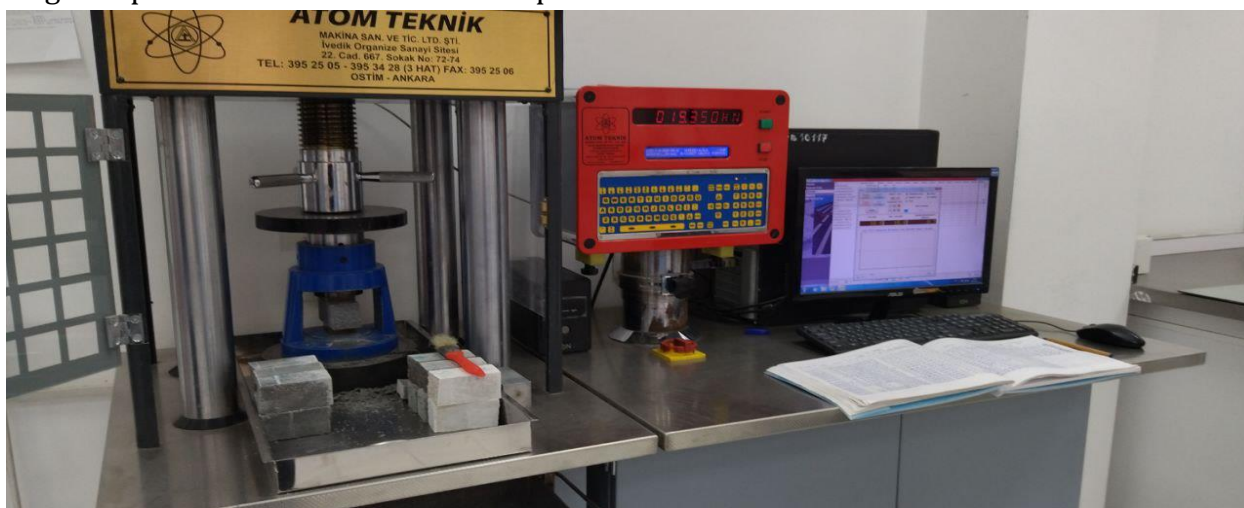
4-picture. To examine the strength of cement samples to compression.
