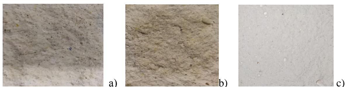
Figure 4. Visual samples of plaster layers formed by solid conglomerate alloy: a - 5%, b - 2% bio-filler and c - samples made of ordinary perlite
