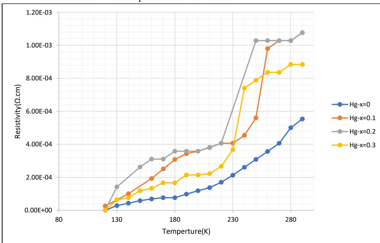
Figure (3) shows the change in electrical resistivity as a function of temperature for the group samples.
