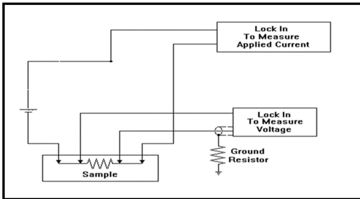
Figure (1). Circuit diagram of the resistivity measurement
