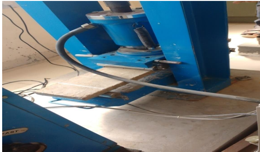
Fig. 4 - Flexural test on Specimens
