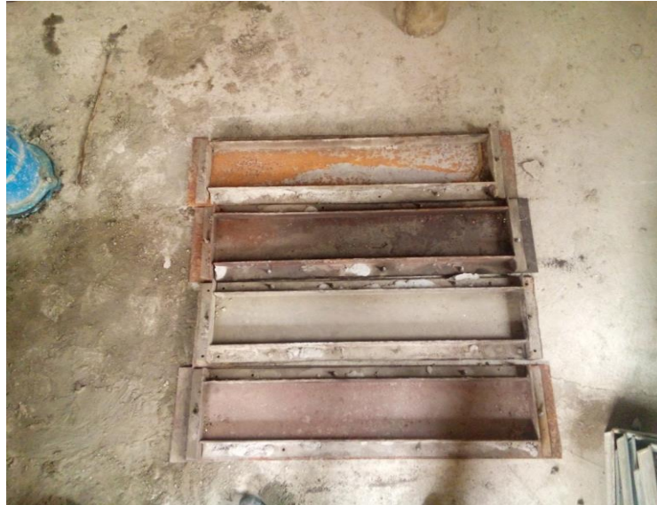
Fig. 3 - Flexure Test Mould
