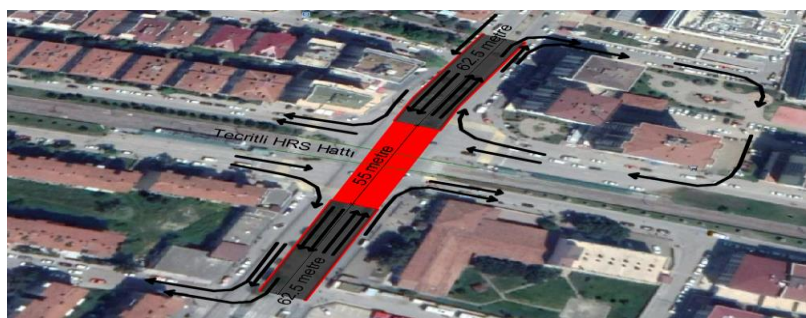
Fig. 3. Türkiş Highway Underpass Model
