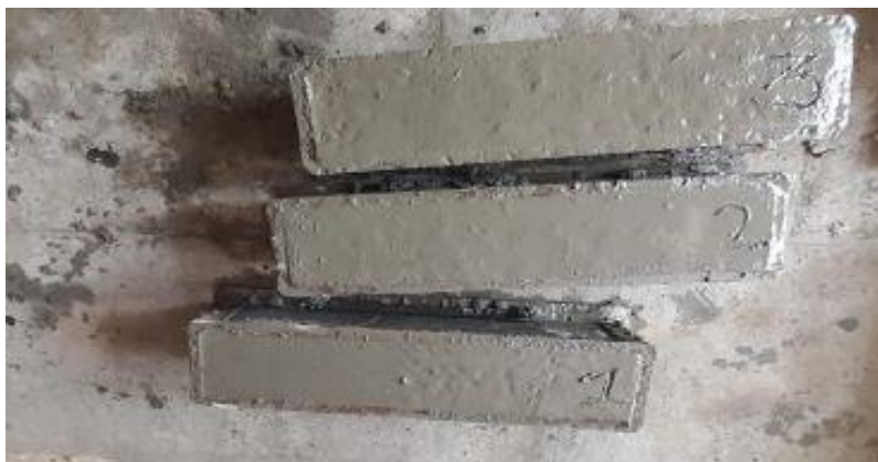
Photograph No 4: Beam after compaction
