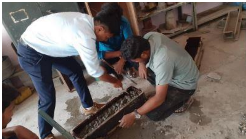
Photograph No 3: Casting of Beam
