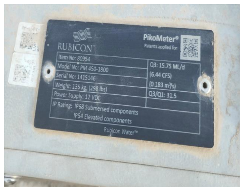
Figure 1. Parameters of the "Rubicon Water" device installed in the Qamashi-Mirishkor canal
