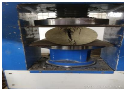
Fig 20 split tensile strength test for different SCC mixes using UTM
