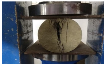
FIG 22 Failure of Cylinder
