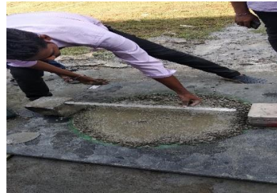
Fig 10 Measurement of slump flow
