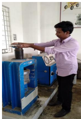
Fig 19 Compressive strength of different SCC mixes using CTM
