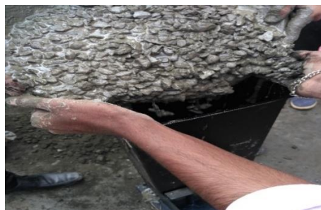
Fig 17 Conducting L-BOX test as per EFNARC guidelines
