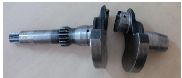
Fig. 1 Final failure On fillet of crankshaft
