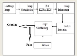
Figure a):- block diagram
