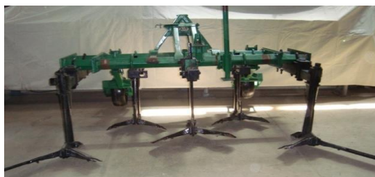
Fig.1. Cultivator-loosener of vineyards UK-3 on cultivation works of row-spacings by processing of inter-bushes lines
