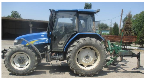
Fig. 2. Cultivator-loosener for vineyards UK-3 for using row-spacings cultivation activities with inter-bushes lines tillage at assembly of the tractor TL-100 "NEW Holland"
