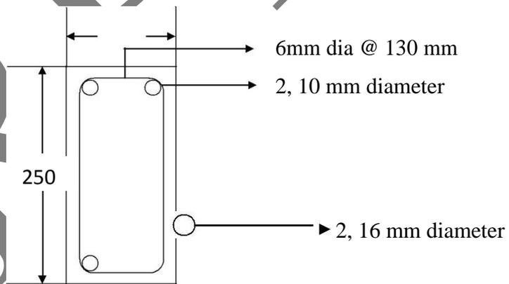
Figure 2: Reinforcement Detailing of Beam
