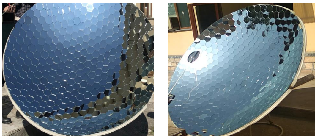
Picture 1. "Solar oven" device: quartz mirrored reflectors.
