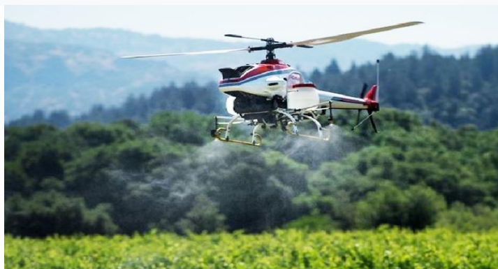
Fig. 2. Yamaha RMAX sprayer on an agricultural field.
