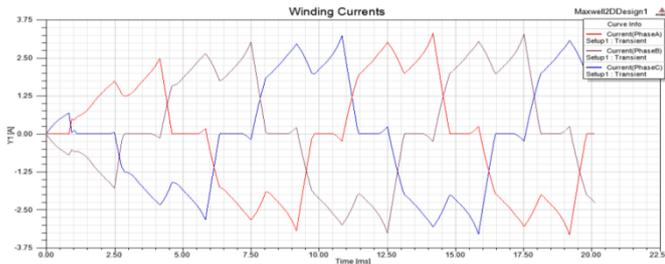
**Fig. 18. Motor winding currents**
