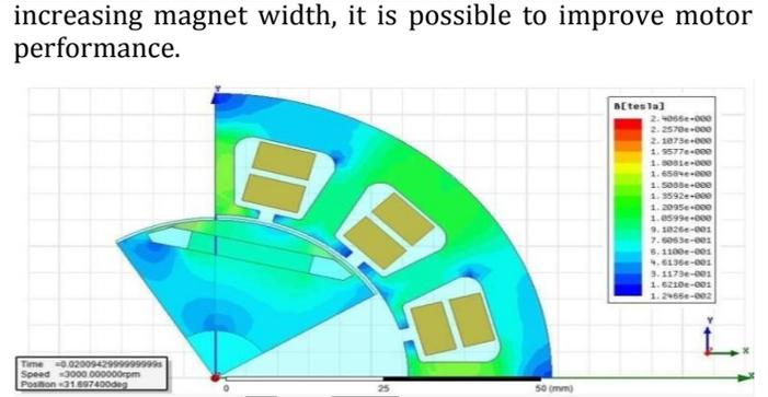
**Fig. 16. Flux density in stator and rotor when rotor is moved**
