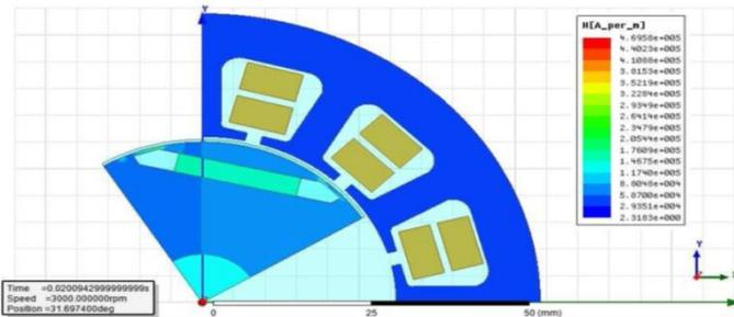
**Fig. 15. Field Intensity in stator and rotor when rotor is moved**
