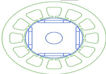
Fig. 7. Cross section view of motor
