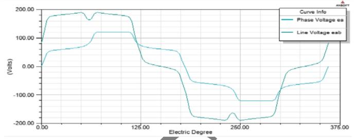
Fig. 12. Plot showing Induced coil voltages
