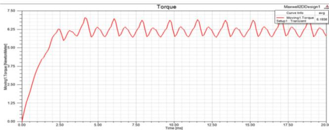
**Fig. 19. Torque output of motor when magnet width is increased**
