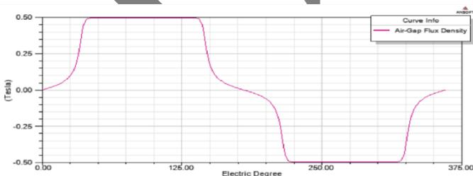
Fig. 11. Plot showing air gap flux density
