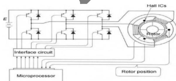
Fig. 1. Schematic of a BLDC motor [3]
