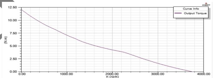
Fig. 9. Plot showing Torque v/s speed
