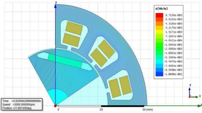
**Fig. 14. Flux lines in stator and rotor when rotor is moved**
