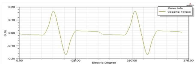
Fig. 10. Plot showing Cogging torque in two teeth
