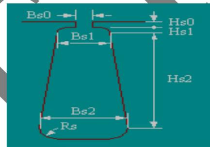
Fig. 3. Slot Dimensions
