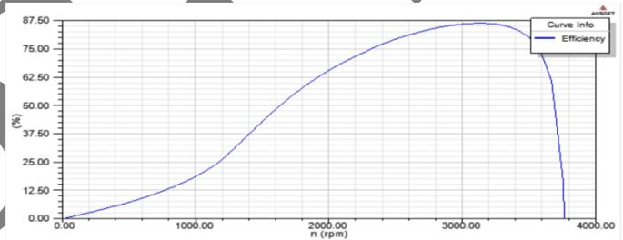
Fig. 8. Plot showing efficiency v/s speed
